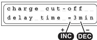
At the start of the charge process the unit initiates a delay time which suppresses automatic charge termination during this (delay) period. This means: during this delay period the charge voltage is **not monitored**, and the battery is charged for at least the set length of time! The charge termination delay is only effective in the NiCd and NiMH charge programs.
