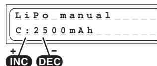
This program charges the battery using the capacity-charge current which you set.
