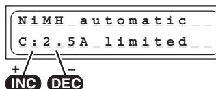
In this program the charger detects the types of battery connected and adjusts the charge current accordingly, to avoid overcharging the pack.
